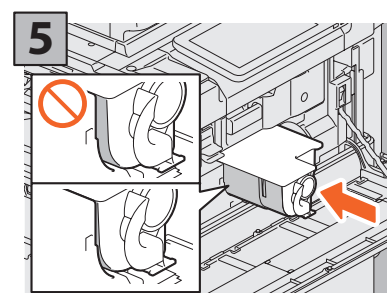
Insert the new toner cartridge until its front surface aligns to the left side wall.
